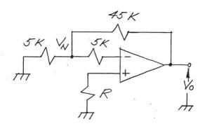
(20pts) 5. The op-amp is ideal except that it has bias currents of 100nA directed into the amplifier. R is chosen to make  $V_0 = 0$ . What are the values of  $V_N$  and R?
